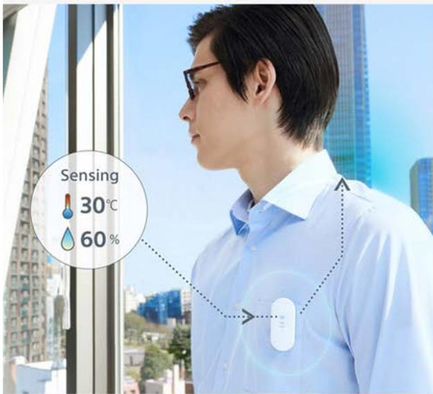
By connecting the newly developed REON POCKET TAG (RNPT-1) with REON POCKET 3 (RNP-3) or REON POCKET 4 (RNP4-4T), the TAG's built-in sensor detects the ambient temperature and humidity, to automatically adjust REON POCKET\*<sup>1</sup> to the temperature level that suits the environment.
